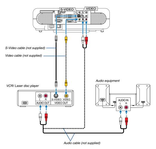
Use an RCA or S-Video cable (not provided) to connect the video and use RCA cables (not provided) to connect the audio from your VCR, laser disc player or document camera to your projector.
